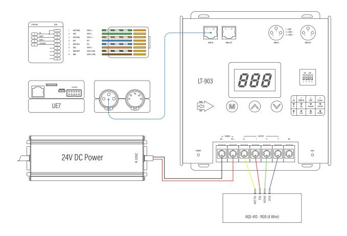
Setup allows for app control (needs to be on a wifi network), calender scene triggers, operation from control systems and scene triggering from external sources. 12 and 24 channel receivers also available. Receivers can be daisy chained. Up to 170 individual runs of neon flex per DMX universe with the appropriate amount of receivers. Up to 2 DMX Universes. Wall Controller also available Max 10m strip run for single end feed and 20m double end feed.
