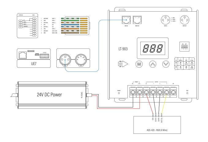
Setup allows for app control (needs to be on a wifi network), calender scene triggers, operation from control systems and scene triggering from external sources. 12 and 24 channel receivers also available. Receivers can be daisy chained. Up to 170 individual runs of neon flex per DMX universe with the appropriate amount of receivers. Up to 2 DMX Universes. Wall Controllers available. Max 10m strip run for single end feed and 20m double end feed.
