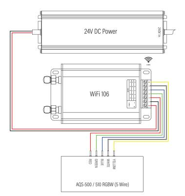
Max 384W 4 channel @ 24VDC. Up to 12 Zones can be controlled from each Wifi-106. 16 Wifi-106's can be run on a Wifi network. RF Range 30m (Line of sight) can be extended with the addition of EBOX-AP's (up to 8 AP's). Max 10m strip run for single end feed and 20m double end feed.
