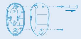
Adjust the system channel to match the selected system channel on the AQR-002 reciever unit. Refit the back cover.
