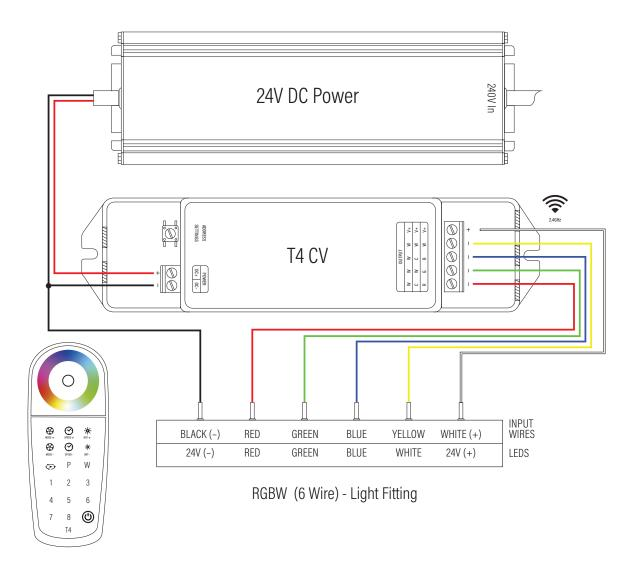
Wireless 4 channel with zoning. Max 480W 4 channel @ 24VDC. Up to 8 Zones can be controlled from T4 Remote. RF Range 30m (Line of sight). Unlimited numbers of T4CV's can be added on each zone. For installations with a load greater than the controller/receiver capacity, the yellow V + wire can be wired directly to the positive + wire from the power supply which can allow up to 600W using a HLG-600H-24 power supply.
