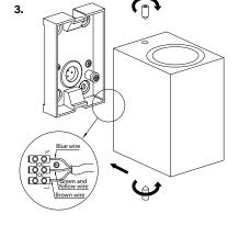
O-Ring must be under washer, No reverse position
