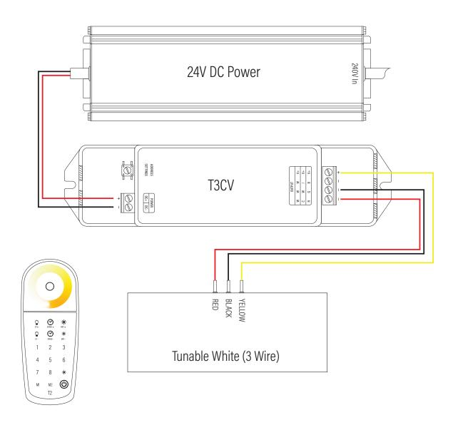
Wireless 2 channel CT setup with zoning. Max 432W 3 channel @ 24VDC. Up to 8 zones can be controlled from T2M remote. RF Range 30m (Line of sight). Unlimited numbers of T3CV's can be added to each zone. Max 5m strip run for single end feed.
